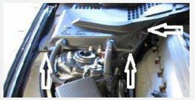
Remove the (3) pin screws that hold the battery cover to the chassis. Disconnect the negative battery terminal.
